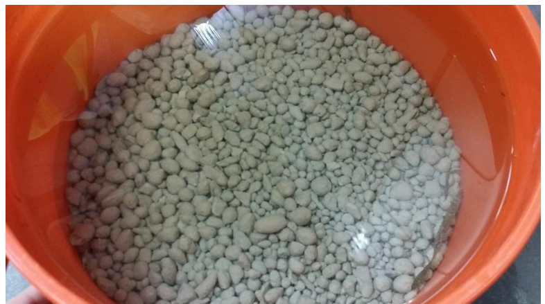
One of the sample buckets, removed from the river post-placement, showing the as-placed AquaGate+Organoclay.
