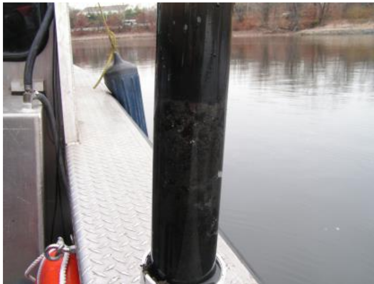
Core sample of mixed layer showing uniform distribution of AquaGate+PAC within capping layer and achievement of target cap thickness
