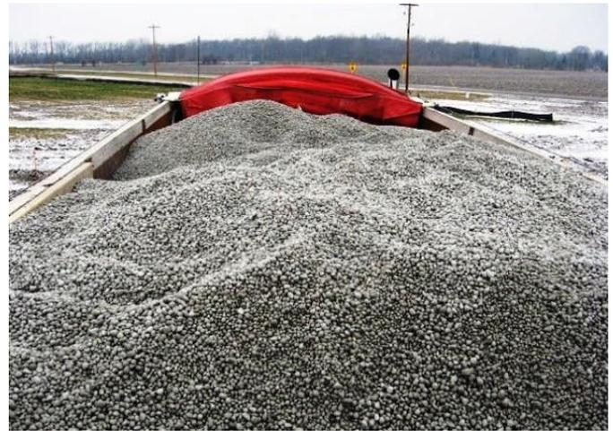
Photo 3. The slinger truck bed/hopper fully loaded with product; capacity typically ranges from 15 to 18 cubic yards (18-22 tons of AquaBlok)
