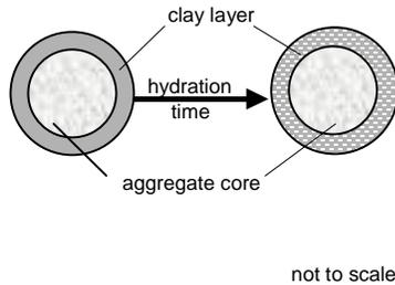
Figure 1. Configuration of Typical AquaBlok Particle.
