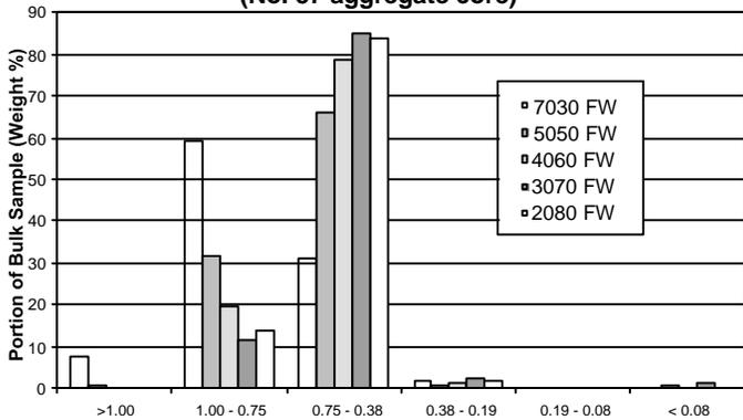
**Figure 4. Relative Bentonite Content (No. 57 aggregate core)**
