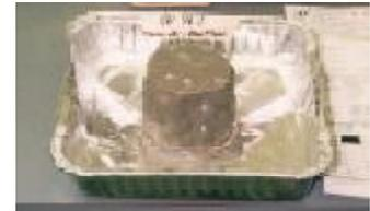
**Photo 2.** Typical AquaBlok sample after permeability testing.
