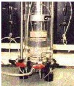
**Photo 1.** Permeability testing of AquaBlok samples.
