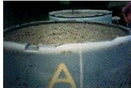
Photo 2. Hydrated AquaBlok prior to instrument installation
