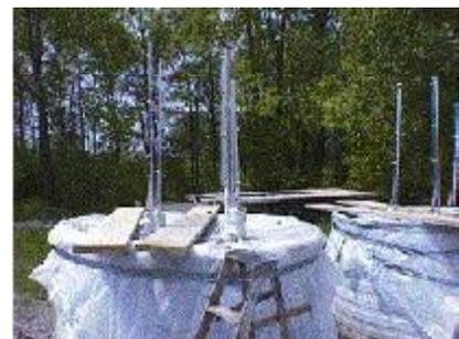
Photo 3. Instrumented Boutwell testing vessels
