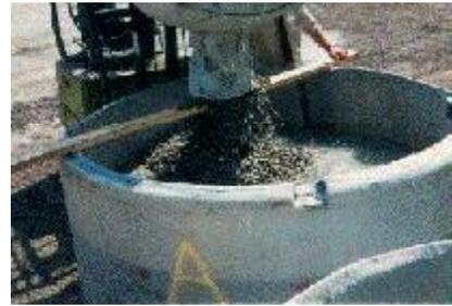
Photo 1. Addition of AquaBlok to testing vessels
