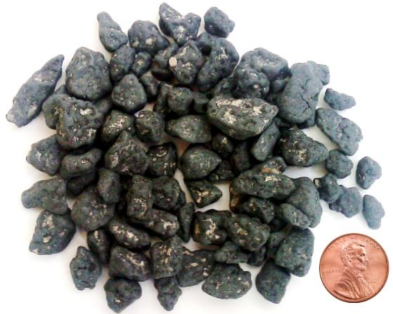
Figure 1. Configuration of PAC-coated particle.
