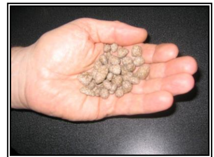
Figure 4. AquaBlok HoleBlok+™ and HoleBlok+™ grout particles are easy to handle and place. No mixing or special equipment is required.
