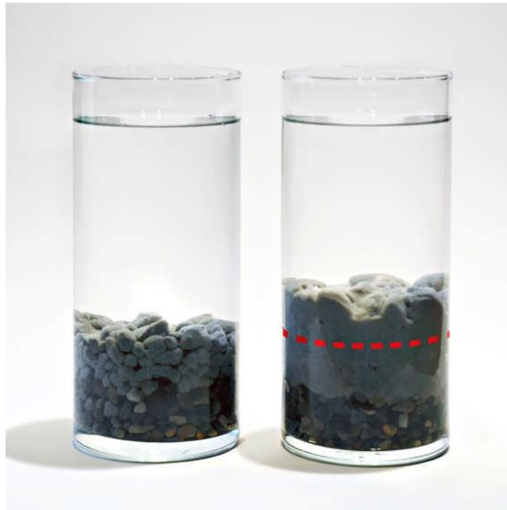
Figure 1. AquaBlok ® applied at 7-lbs/ft 2 (~1” dry material thickness) atop ~1” layer of ordinary gravel. Time lapse: LEFT: immediately after inundation and RIGHT: 24 hours after inundation. Note original boundary between product and water (dashed red line) demonstrating swell/expansion of product over time.
