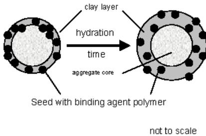
**Figure 1. Configuration of Typical SubmerSeed® Particle.**
