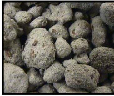
**Photograph 1. Close-up of typical SubmerSeed particles (approximate size: ¼ - ½")**
