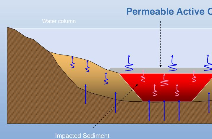
Figure 1: Graphic of Conventional Permeable Active Capping Layer
