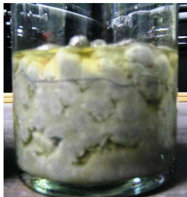
Photo 1. Example Design Mix – 300g of AquaGate+ORGANOCLAY 4060 blend sample (120g of Active Organoclay), 3 weeks after addition of 185ml motor oil.
