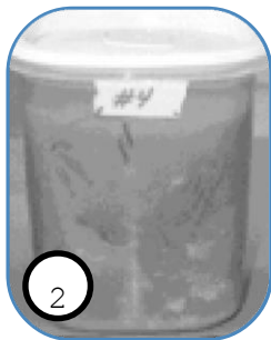
Representative test sample after third freezing event – Note fractures.
