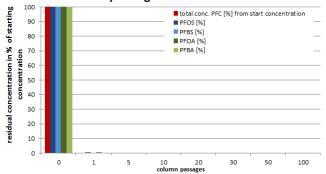
Figure 1: Residual PFC concentrations (% of starting concentration) after 0, 1, 5, 10, 20, 30, 50 and 100 column pore volumes of RemBind Plus
